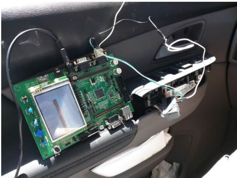
Figure 5: RV-ECU development prototype connected to the body CAN bus of a 2012 Honda Odyssey
